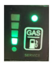
• if running on LPG, when LPG runs out the vehicle will beep then switch seamlessly back to petrol
