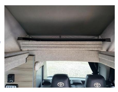
To lower the roof, firstly lay the boards flat again (otherwise the roof won't lower properly and you will put too much pressure on the struts) then pull the handles down, pull the fabric in (so it is not trapped outside) and secure with the two straps tightly before moving off.
