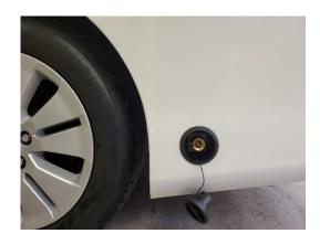
When adaptor and hose are attached correctly, press fill button, the pump will cut out when the tank is full (LPG tanks fill to 85% so expect approximately 65L when filling from empty). Release the hose attachment (expecting excess gas to be released) and fully detach. Replace black LPG cap.
